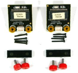
The ICE can only be purchased as a kit: CY3215-DK. In addition, if you are using QFN packages an Emulation Kit (CY3250-xxxx-QFN) must be purchased for adapting the specific package to the POD. The package you choose can be adapted to any POD with a "Foot," or package adapter. Detailed selection guides follow in the appendix.
