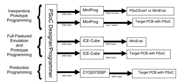
\* This friction-lock 5-pin header that connects target PCB to Miniprog can be ordered as DigiKey WM4203-ND.
